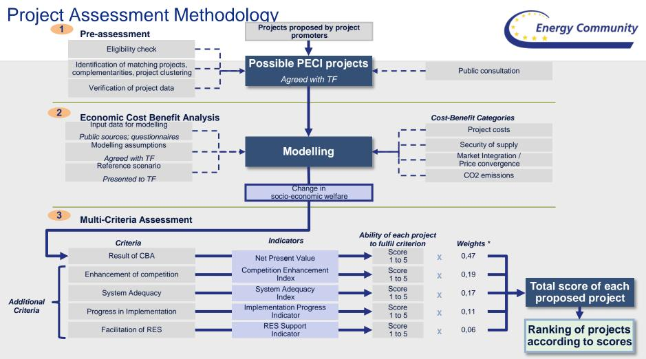
\* Weights and criteria differ slightly for the different groups (electricity infrastructure, electricity generation and gas infrastructure). In this graph criteria and weights for electricity generation are presented.
