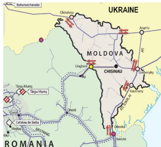
Figure 57. Regional interconnection points of the gas transport system of the RM
