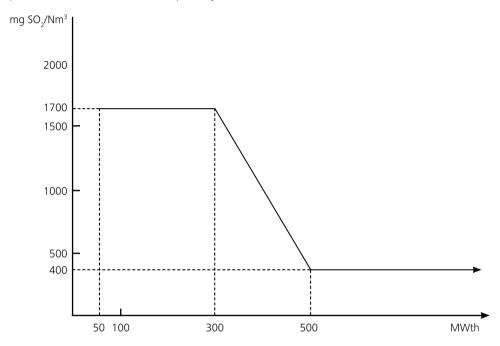
B.  $SO_2$  emission limit values expressed in mg/Nm<sup>3</sup> ( $O_2$  content 3%) to be applied by new plants pursuant to Article 4(2) with the exception of gas turbines
