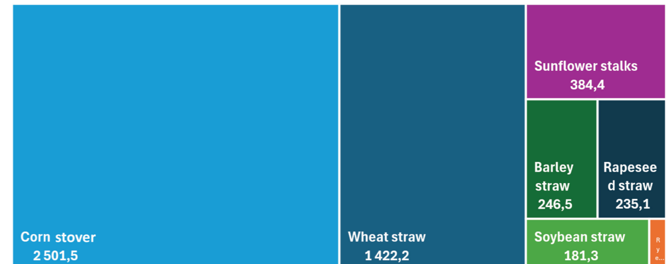
Fig. 10.1 – The structure of biomethane production potential from crop residues in Ukraine (mIn Nm 3 CH 4 /yr)
