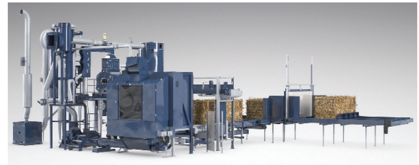
Fig 5.7 – LinKa and Euromilling mini-complex for specialized straw milling
