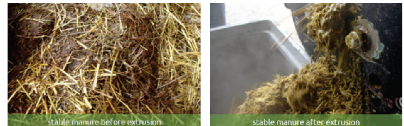
Fig. 5.8 – Cattle manure before and after processing in a bioextruder
