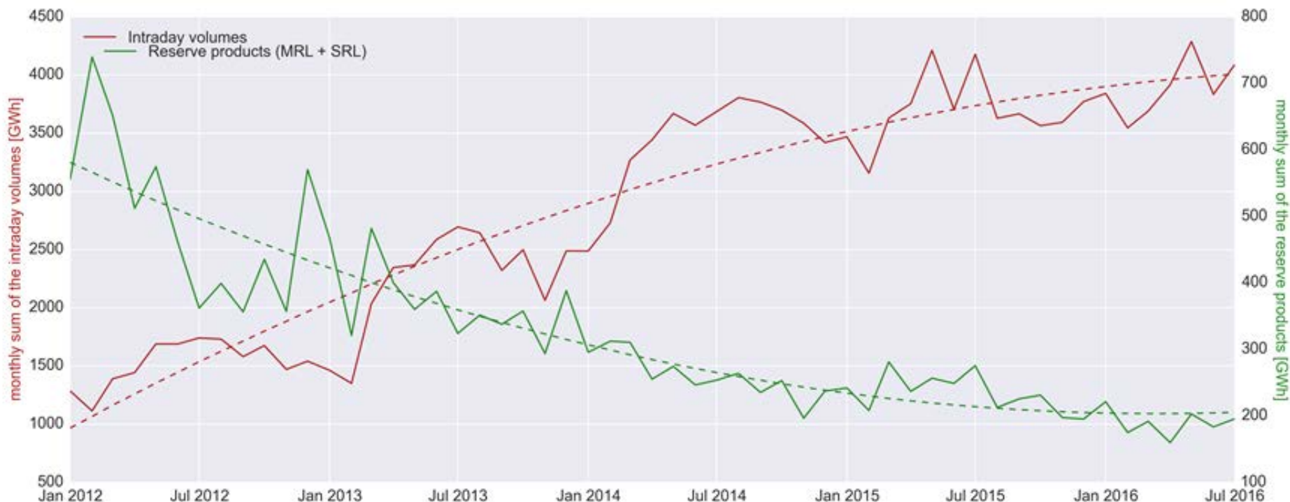
Graph: Volumes in the activated reserve markets (green) versus intraday market (red) in Germany
