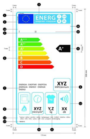
4.3. For gas fired household tumble driers, the design of the label shall be as in the figure below.
