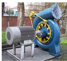
Exterior view of a Francis turbine attached to a generator (source: Wikimedia Commons CC BY-SA 3.0)
