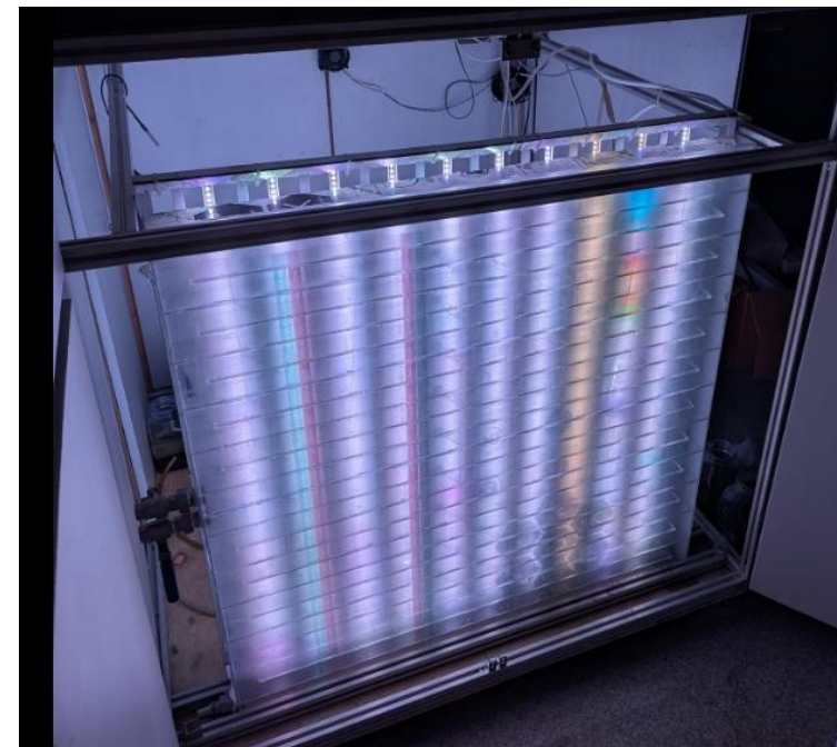
Flat-plate PBR made of polycarbonate sheet
