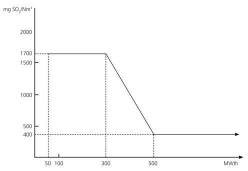
B.  $SO_2$  emission limit values expressed in mg/Nm³ ( $O_2$  content 3%) to be applied by new plants pursuant to Article 4(2) with the exception of gas turbines
