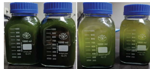
Fig. 2.11 - Natural sedimentation of Chlorella vulgaris (Photo by the authors of the AN)
