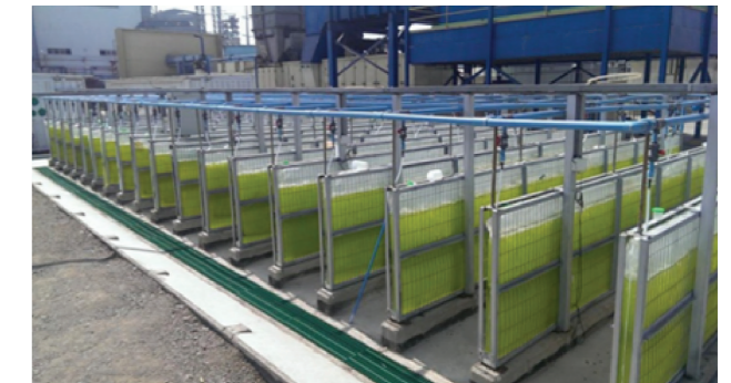
Fig. 2.4 - Pilot flat-panel photobioreactor system (1.5 m height, 10 m length, 0.10 m width), located in Tocopilla, Chile, at the E-CL power station 71
