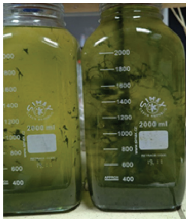
Fig. 2.8 - Chemical flocculation in laboratory conditions using Chitosan (Photo by the authors AN)
