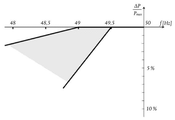
The diagram represents the boundaries in which the capability can be specified by the relevant TSO.
