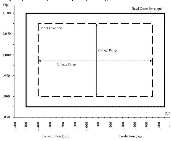
The diagram represents boundaries of a U-Q/ $P_{max}$ -profile by the voltage at the connection point, expressed by the ratio of its actual value and the reference 1 pu value, against the ratio of the reactive power (Q) and the maximum capacity ( $P_{max}$ ). The position, size and shape of the inner envelope are indicative.
