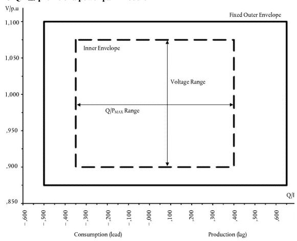
The diagram represents boundaries of a U-Q/ $P_{max}$ -profile by the voltage at the connection point, expressed by the ratio of its actual value and its reference 1 pu value, against the ratio of the reactive power (Q) and the maximum capacity ( $P_{max}$ ). The position, size and shape of the inner envelope are indicative.
