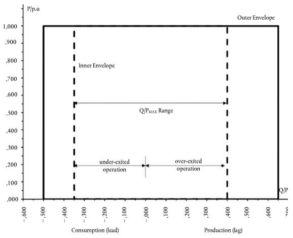
The diagram represents boundaries of a P-Q/P<sub>max</sub>-profile at the connection point by the active power, expressed by the ratio of its actual value and the maximum capacity pu, against the ratio of the reactive power (Q) and the maximum capacity ( $P_{max}$ ). The position, size and shape of the inner envelope are indicative.
