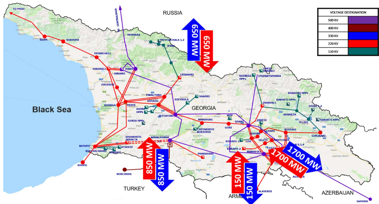
Figure 1. Current [2023] cross-border transfer capacities between the power systems of Georgia and neighbouring countries [11]
